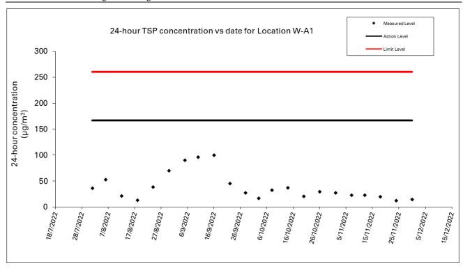
Figure 3: Graphical Illustration of Measured 24-hour TSP (µg/m³) Levels at W-A1
