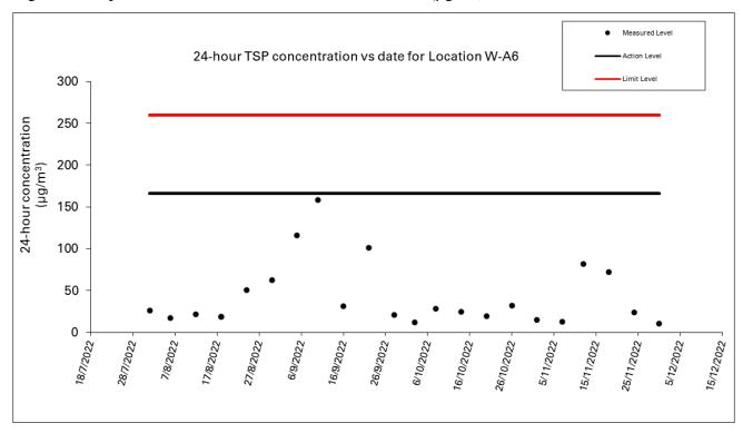
Figure 4: Graphical Illustration of Measured 24-hour TSP ( $\mu g/m^3$ ) Levels at W-A6
